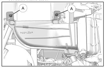
2. Remove one screw from side of plenum.
