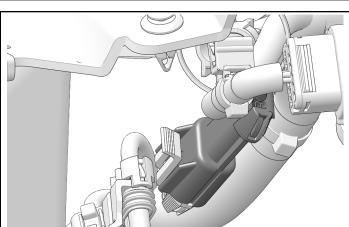
11. Use one cable tie ② to bundle extra length of RCA power wire and attach to main vehicle harness.
