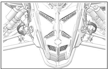
3. Turn hood fasteners clockwise to lock hood.
