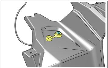
3. **Axys models:** Connect RCA power wire connector ① to vehicle harness connector ⑩ in fabric bag.
