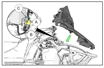
Turn two hood latch fasteners at rear corners of hood
