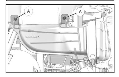
5. Install one screw on side of plenum.
