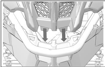
2. Pull sides of hood out and install over side panel fasteners.
