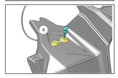
2. Push/pull remaining portion of plug into grommet until it is flush with the end, as shown.
