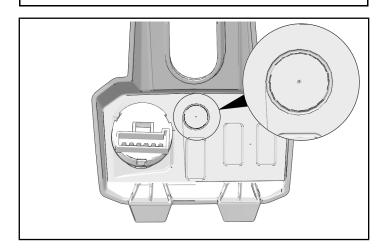
6. Route RCA plug ① through opening. Fit grommet over RCA plug and into hole.
