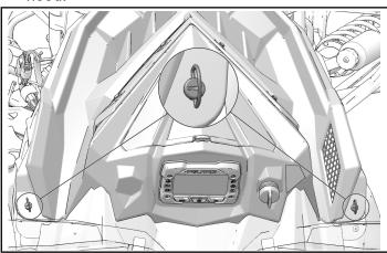
3. Slightly lift rear of hood and disconnect hood harness (a) from main chassis harness (b). Cut cable tie (c) attaching hood harness to chassis, if applicable.
