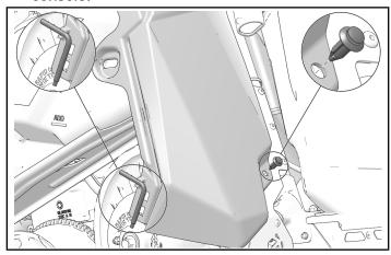
3. Install two dart clips on right side of console.
