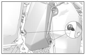
2. Remove clutch tool and dart clip from left side of console.
