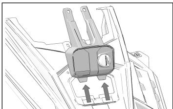
4. Remove plastic nut from tether switch (if equipped). Remove tether from switch panel and re-install plastic nut.
