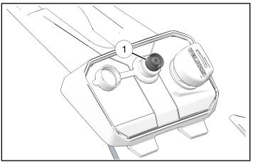
8. Install tether switch (if equipped). Remove plastic nut from tether and install in switch panel. Install plastic nut.
