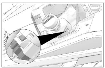
10. Locate power connection on right side of snowmobile. Vehicle connector will be labeled "RCA plug." Remove protective cap and connect RCA power wire.
