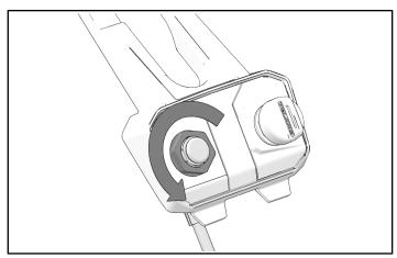
5. Center hole saw on witness mark. Use hole saw to cut out opening.
