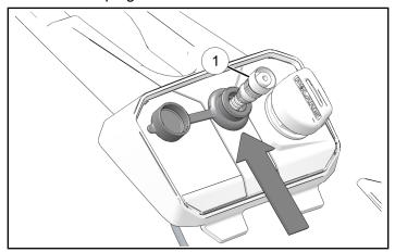
7. Install RCA plug 1 until it is seated in grommet.
