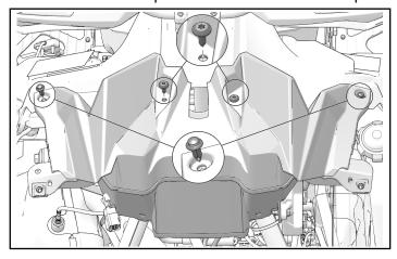
5. Lift off and set aside upper intake plenum.
