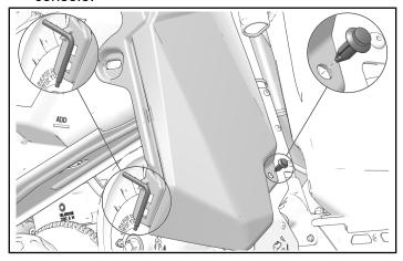
3. Slide console rearward slightly. Disconnect console switch harness from chassis harness.
