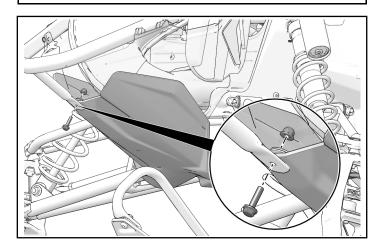
6. Locate three pre-existing holes at front of tunnel.
