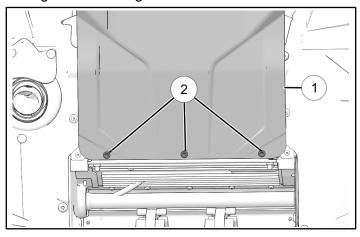
8. Loosely install two front bumper screws.
