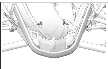
9. Torque five bumper fasteners to specification.
