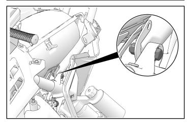
3. Remove and keep two screws holding the left and right hand side of bumper to the nose pan.
