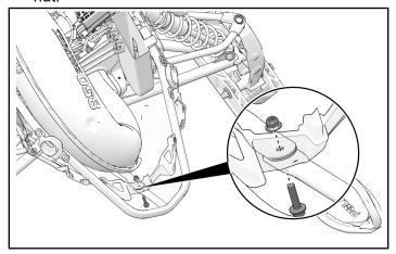
5. Put Sentry Skid Plate under the front bumper mounting tab as shown. Insert the original center bumper mounting bolt and loosely install kept nut.
