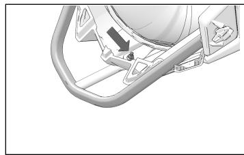
10. Install spring connecting tuned exhaust pipe to bumper.
