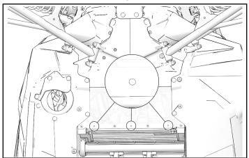
7. Align skid plate with three pre-existing holes. Attach rear of skid plate ① using three screws ②. Tighten until snug.
