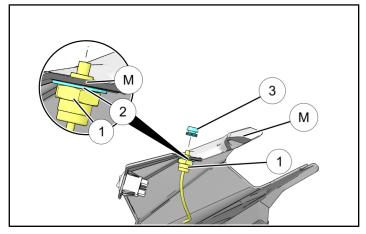
f. Next, locate the fabric bag ® covering the electrical connections in the area indicated. Open the bag and locate the male two pin powered accessory plug ① that will connect to the tether switch and remove the protective cover ① as shown.
