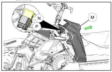
The console should now be in a position to allow you to drill the tether switch mounting hole in the following steps.
