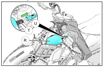
g. Locate the female connector of the tether ③ and connect with the male end on the chassis harness ①. Once connected, close the electrical cover bag over the connections.
