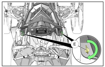
b. After installing hood, install both side panels making sure all latches and rubber straps are fully secured.
