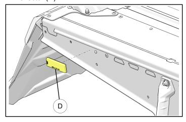
3. Clean extreme rear bumper ① sides with Isopropyl alcohol or other suitable cleaner/degreaser. Install new reflector ② on rear bumper ①.
