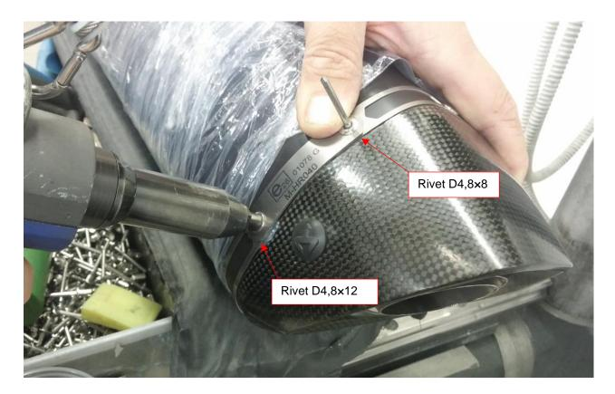
4. Step: After riveting make sure you wipe off excessive silicone. Remove the wrapping.
