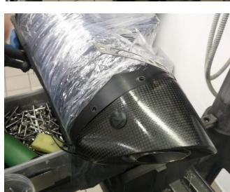
2. Step: Fill the holes with silicone on both sides
