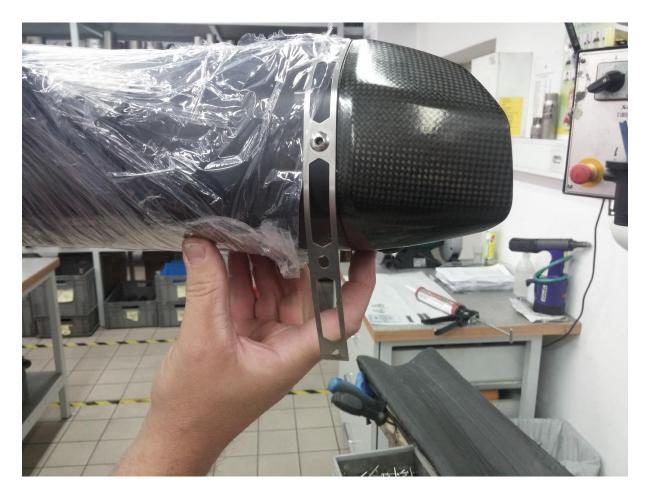
After applying silicone in both holes, turn muffler around and make sure that the remains of the rivets stick to it.
